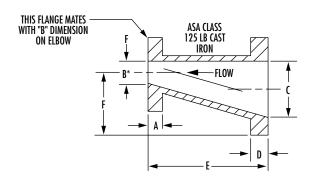
Eccentric suction increasers are optionally available for use on Models 612A, 613A and 614A pumps in conjunction with suction elbows. Larger suction line diameters are easily accommodated by these combined options. (Example: A pump with 8" (203) suction can be connected to a 12" (305) suction line by using an 8" x 10" (203 x 254) suction increasing elbow and a 10" x 12" (254 x 305) eccentric suction increaser.
