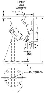
[4]-7/8 (22) DIA. HOLES ON 11-3/4 (298) DIA. BOLT CIRCLE. STRADDLE CENTERLINES
