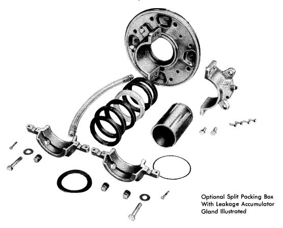
Split packing boxes separate vertically through the packing insert to simplify packing replacement and shaft sleeve inspection. The insert halves are dowled, register aligned and gasketed to prevent leakage. Only six bolts need be removed to expose all of the packing and lantern ring. Remove two more bolts and the remaining packing box insert half can be removed.
