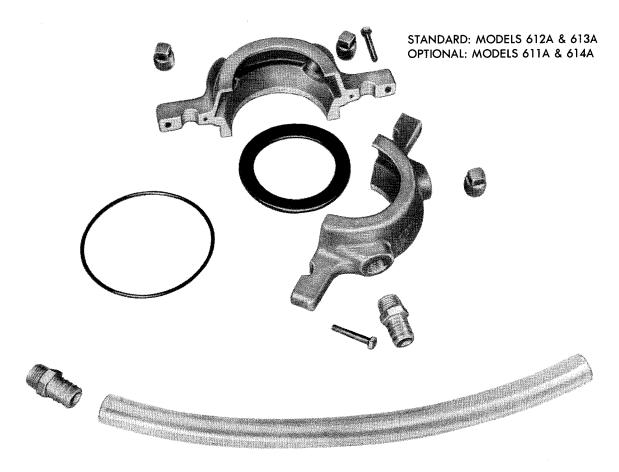
The leakage accumulator gland (sprayless, dripless packing gland) is designed and constructed to prevent the collection of packing leakage in the pump bracket of a vertical or horizontally mounted pump. The leakage accumulator gland has a volute shape with two symetrical halves. This gland encloses the water slinger preventing any spray from escaping and contaminating the area. The leakage is efficiently directed to a drain connection.
