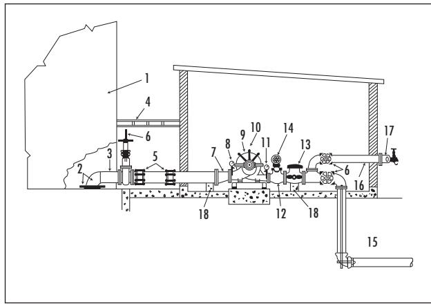
**ARRANGEMENT OF CENTRIFUGAL FIRE PUMP WITH WATER ALWAYS UNDER A HEAD**
