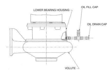
THE OIL CHAMBER FILL/DRAIN DEVICE IS NOT UL APPROVED. USE OF THIS DEVICE WILL VOID THE UL LISTING ON THE MOTOR.
